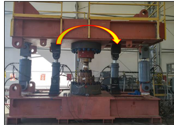
External Load and Hub Separation tests
