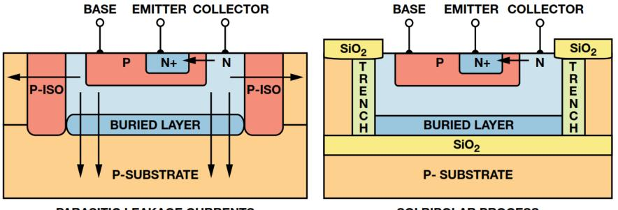
PARASITIC LEAKAGE CURRENTS ON TYPICAL BIPOLAR PROCESS SOI BIPOLAR PROCESS
