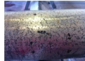
Halide brine corrosion damage W. Canadian examples
