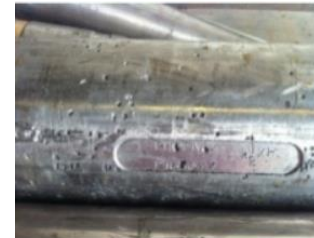
Halide brine corrosion damage W. Canadian examples
