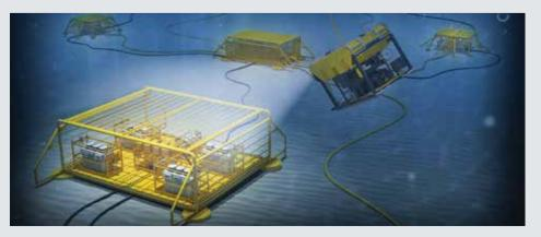
**FIG. 1.** ABB is developing reliable power sources to operate in water depths of 3,000 m, and over distances up to 600 km.
