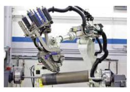
**FIG. 1.** The AFP manufacturing method, creating a composite structure using continuous fiber-tape. Image: Trelleborg Offshore.
